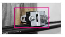
**SUSPENSION GROOVED PADS.** This technology is used for figure-8 cables with steel or dielectric messenger. Designed with two grooves to adapt to different messenger diameters. Available for fixed or mobile suspension applications.
